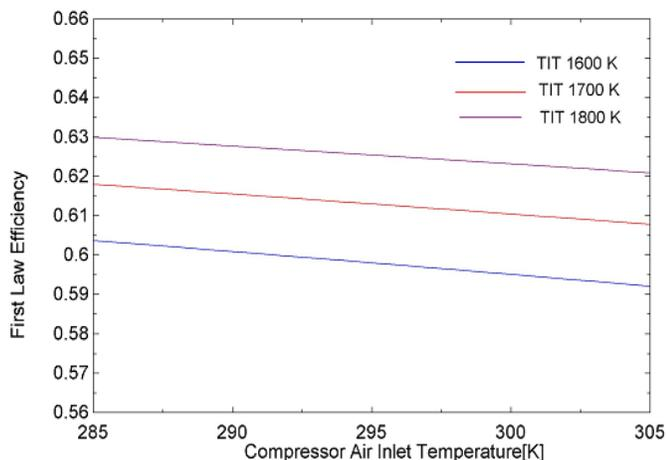
Figure 24: Effect of compressor inlet air temperature on first law efficiency
