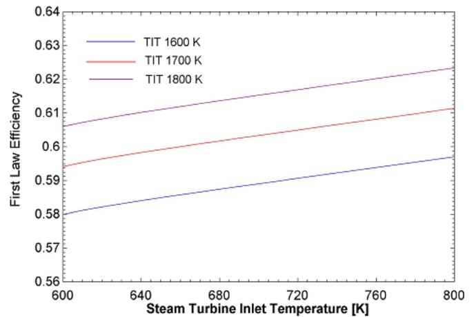
Figure 22: Effect of steam turbine inlet temperature on first law efficiency
