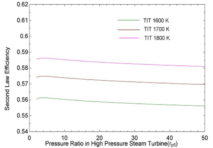
Figure 21: Effect of pressure ratio of high pressure steam turbine on second law efficiency
