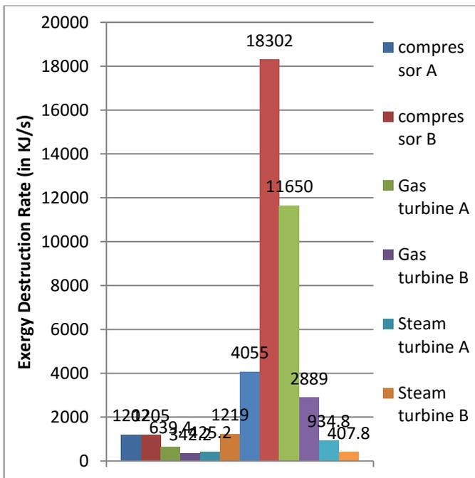
Figure 9: Exergy destruction rate in different components of Modified combined cycle system
