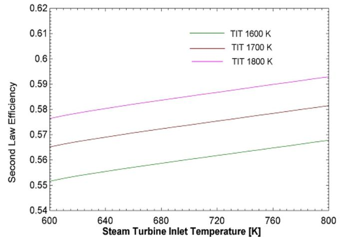
Figure 23: Effect of steam turbine inlet temperature on second law efficiency
