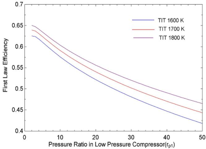
Figure 12: Effect of pressure ratio in low pressure compressor on first law efficiency
