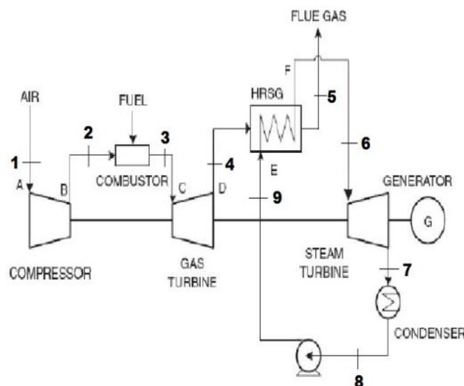
Figure 4: Simple combined cycle gas turbine
