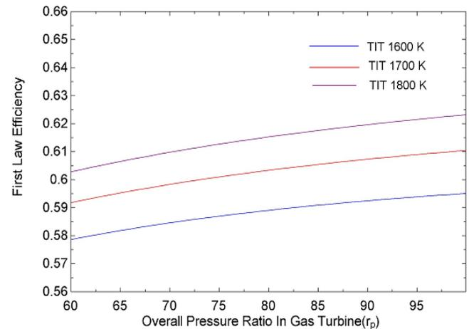
Figure 10: Variation of first law efficiency with overall pressure ratio in gas turbine
