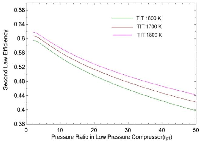
Figure 13: Effect of pressure ratio in low pressure compressor on second law efficiency
