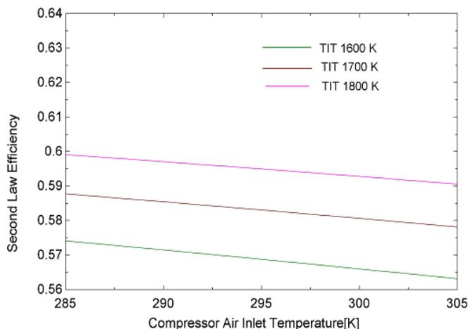
Figure 25: Effect of compressor inlet air temperature on second law efficiency
