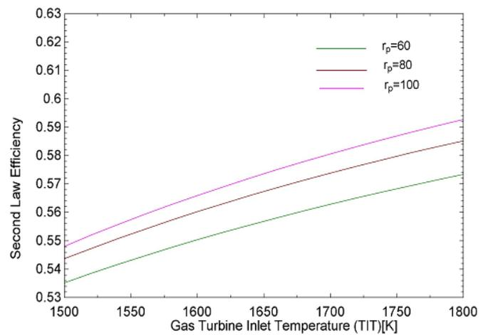
Figure 17: Effect of gas turbine inlet temperature on second law efficiency
