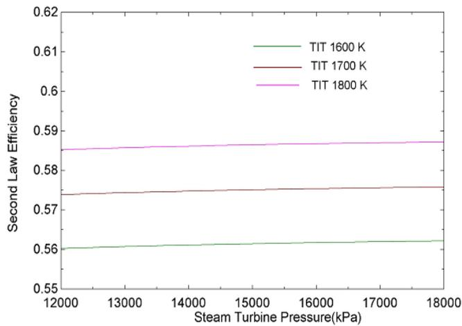
Figure 19: Effect of steam turbine pressure on second law efficiency
