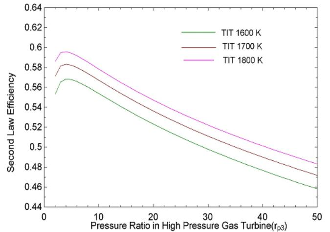
Figure 15: Effect of pressure ratio in high pressure gas turbine on second law efficiency
