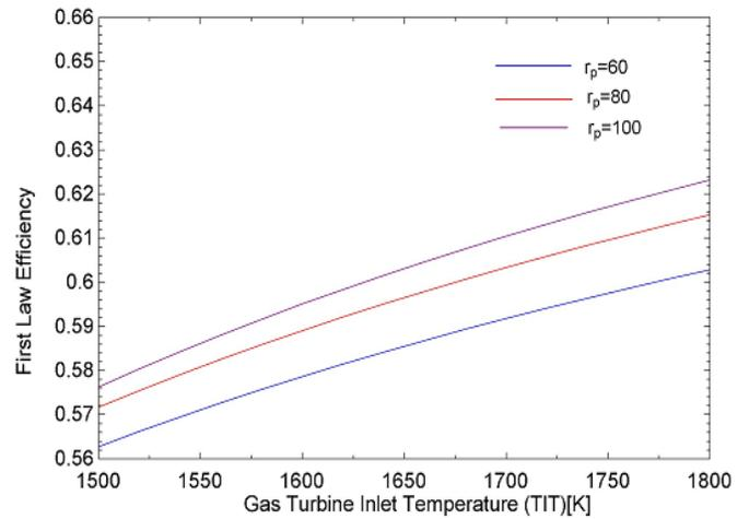
Figure 16: Effect of gas turbine inlet temperature on first law efficiency
