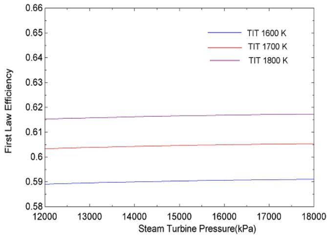
Figure 18: Effect of steam turbine pressure on first law efficiency
