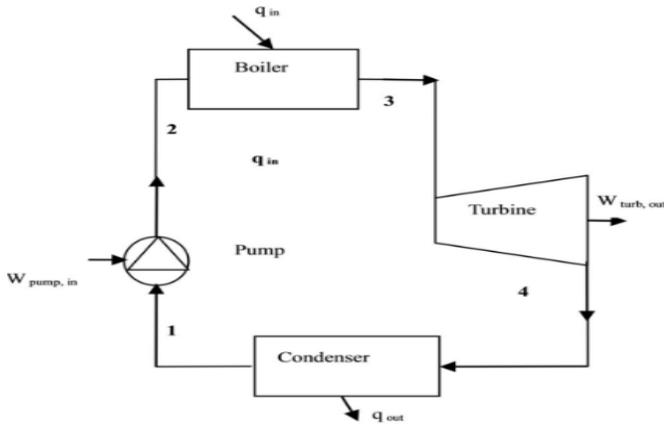
Figure 3: Simple Rankine cycle [2]
