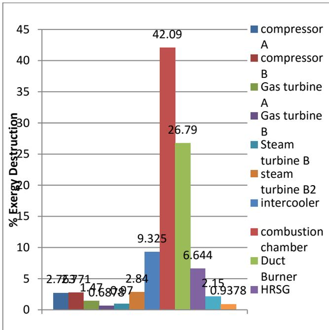
Figure 8: % Exergy destruction of total Exergy destruction in different components of simple Combined Cycle Gas Turbine System
