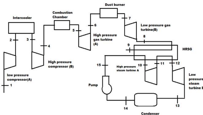
Figure 7: Modified combined cycle system
