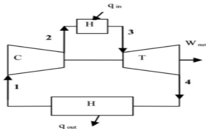
Figure 1. A closed cycle gas turbine [2]
