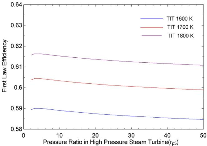
Figure 20: Effect of pressure ratio of high pressure steam turbine on first law efficiency
