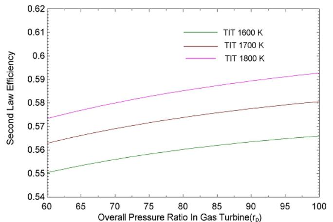
Figure 11: Variation of second law efficiency with overall pressure ratio in gas turbine
