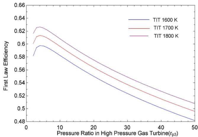
Figure 14: Effect of pressure ratio in high pressure gas turbine on first law efficiency
