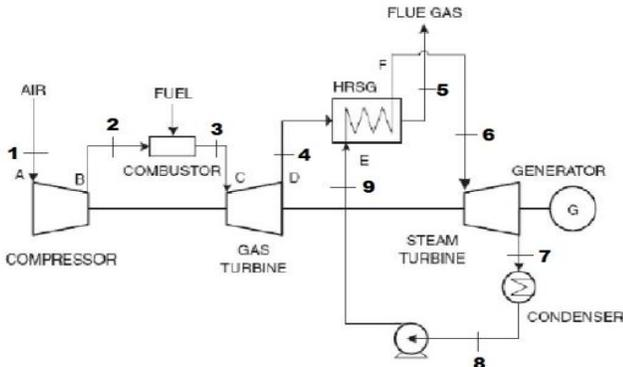
Figure 6: Simple Combined Cycle Gas Turbine System
