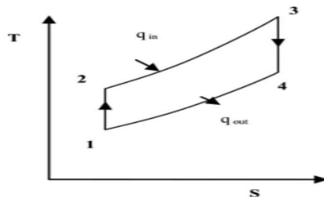
Figure 2: T-s diagram of Brayton cycle [2]
